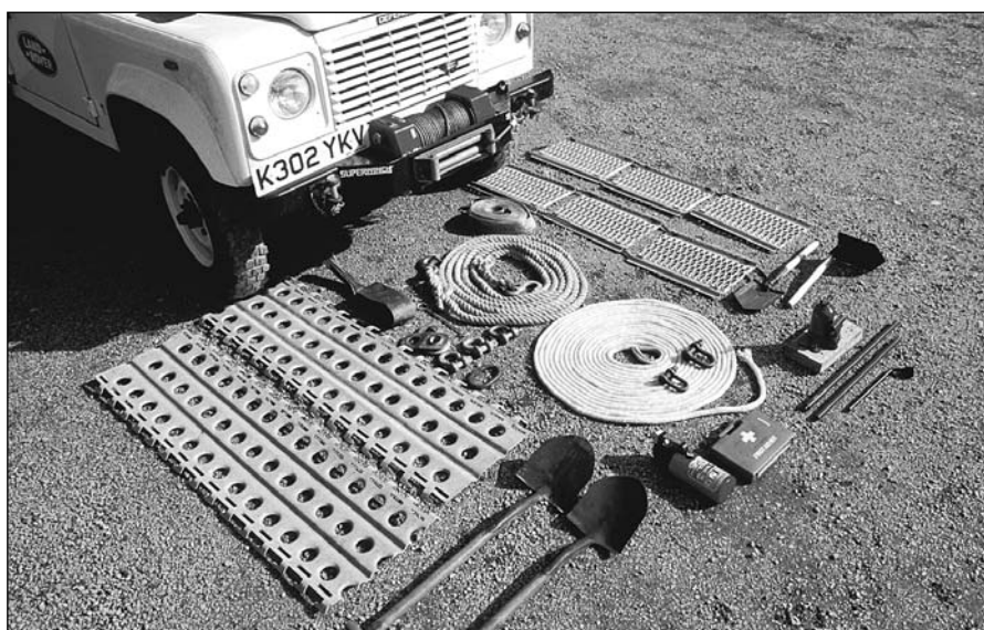
Figure 28.10 Give careful thought to recovery equipment: “sand channels” of some kind to put under the wheels for flotation in slippery mud or soft sand; shovels and long tow ropes so the tug does not get stuck in the same hole as the stricken vehicle. Winches are heavy and expensive; rarely useful except with multi-vehicles in forests or jungle (© Tom Sheppard)
