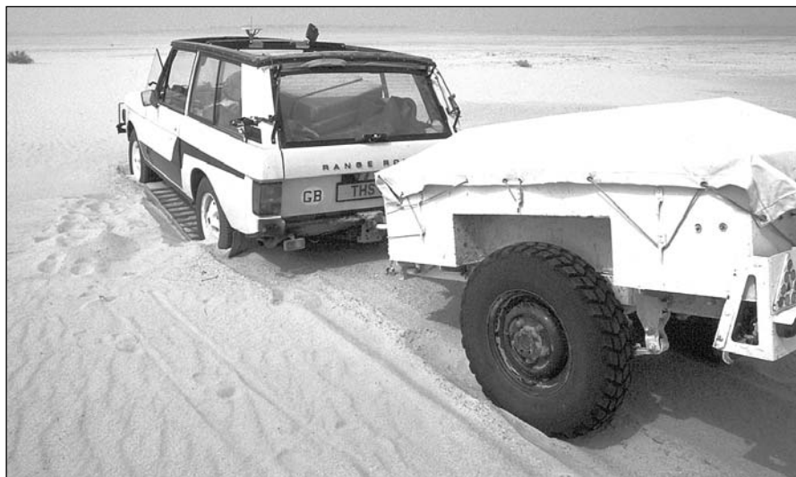
Figure 28.5 Classic example of a fuel-carrier trailer off-loading the main vehicle. Note also how the under-tyred tug has bogged whereas the lightly laden trailer on larger tyres at low pressures rides over the soft sand (© Tom Sheppard)
