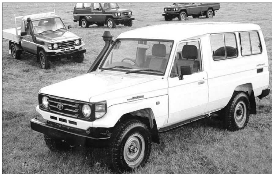
Figure 28.9 Classic robust simplicity – the Australian spec Toyota Type 78 even comes with long-range fuel tanks as standard. This one has coil springs at the front. Never imported into UK, earlier all-leaf-sprung Type 75 in diesel form is highly valued in continental Europe for expedition work (© Tom Sheppard)
