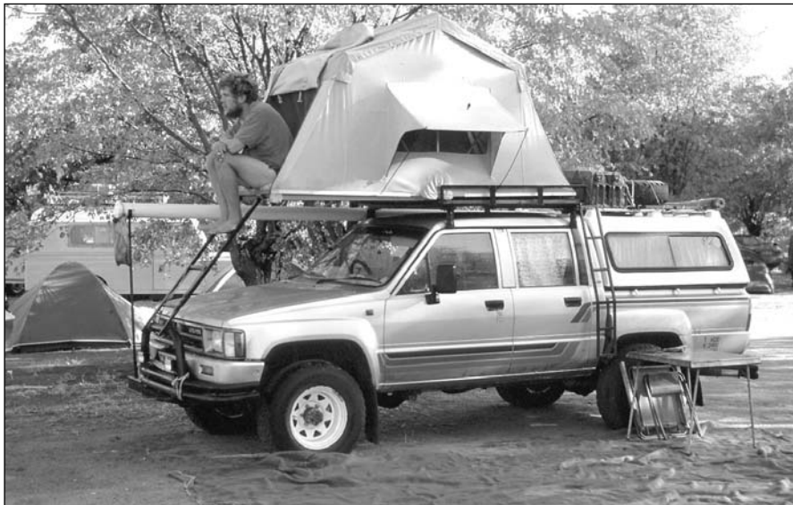
Figure 28.7 Classic application of the crew-cab 4 \times 4 Toyota pickup in short-range expedition role, very popular in South Africa. Note that any heavy cargo will all be over the rear wheels (© Tom Sheppard)
