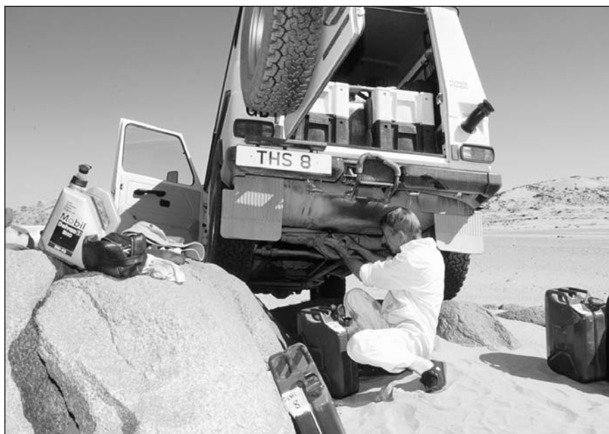
Figure 28.11 Be ready to improvise. Electronic control unit (ECU) defaulting to “limp home” and suspected fuel contamination demanded drain and filter for all fuel on board – an all-day job. Rocks provide handy ramp for jerry can access; failing that a dig-down hole would have sufficed (© Tom Sheppard)
