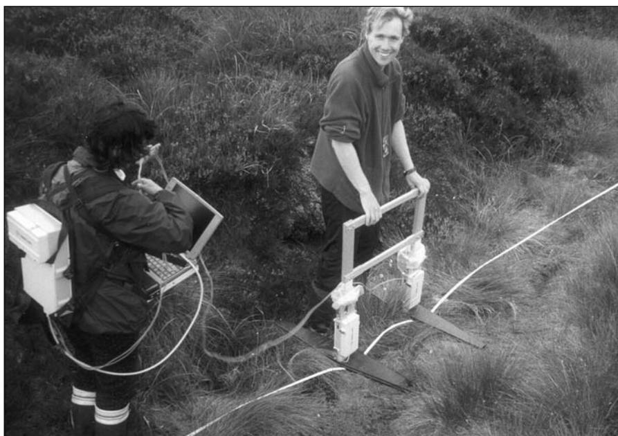
Figure 24.3 *Using ground-penetrating radar to measure soil density in peat. Remember, if you are using sophisticated equipment in wetland environments it is absolutely essential that this is tested thoroughly beforehand and if necessary protected from the wet* (© Jo Holden)
