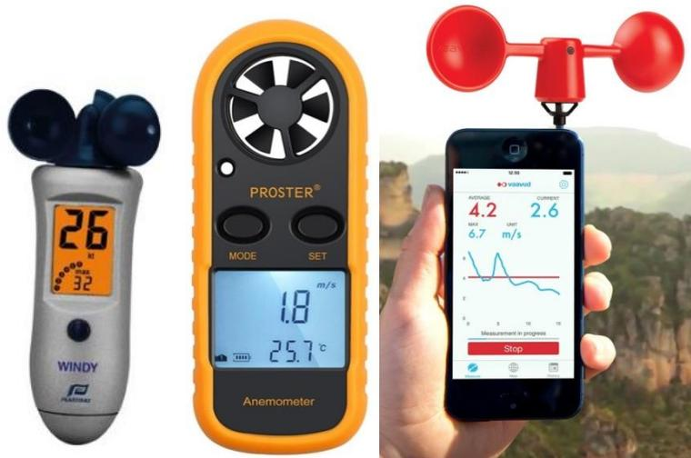
With anemometers, you generally get what you pay for. Cup anemometers (left) are best, because they work whatever direction the wind is coming from. However, they can be expensive and are very delicate. Propeller anemometers (centre) can be much cheaper. However, the propeller has to be pointed into the wind to get a good reading; the wind direction can be hard to judge when the wind is weak or gusty.
