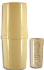
Rainfall is easy to measure using simple, cheap manual rain gauges such as that shown above. The rainfall amount should be recorded at the same time each day, and then emptied. To avoid the gauge being blown over by the wind, it should either be placed in a slight hole in the ground, or partially buried in a flower pot or similar.
