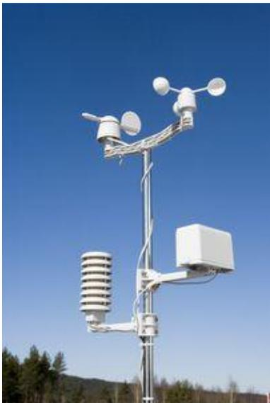
Cheaper automatic weather stations measure many of the same variables as their more expensive counterparts but do not, generally, record information or allow you to upload it to a computer. They usually also suffer from inadequate thermometer shielding, so will tend to overestimate temperatures when the sun is shining onto the station.
