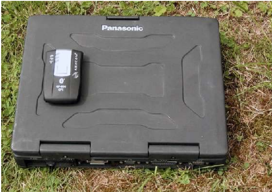
Figure 13-9 Field PC and wireless GPS unit. The GPS shown here has no LCD screen and can communicate wirelessly via blue-tooth. The advantage of this is that the GPS unit can be used in conditions below 0°C. The Panasonic CF-27 can also be used in inhospitable conditions without risk of damage.
