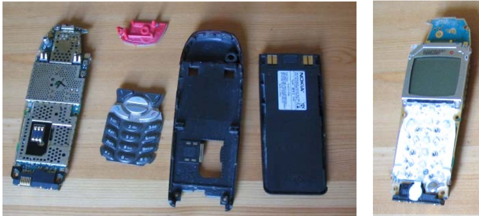
Figure 13-3 Disassembling a mobile phone to prevent water damage.
