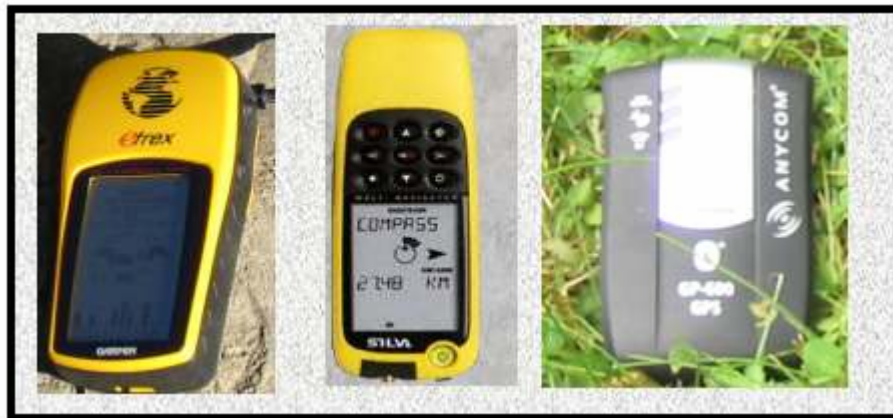
Figure 13-10 GPS Receivers: Basic ETREX, Silva MultNavigator, AnyComm GP600. The ETREX has an operating range of 50°C to 0°C, The Silva 50° to -15°C and the AnyComm 60°C to -20°C. For temperatures beyond this a GPS using an external antenna is the best solution but that requires the unit to be stowed somewhere protected from the elements and generally negates the use of waypoints.
