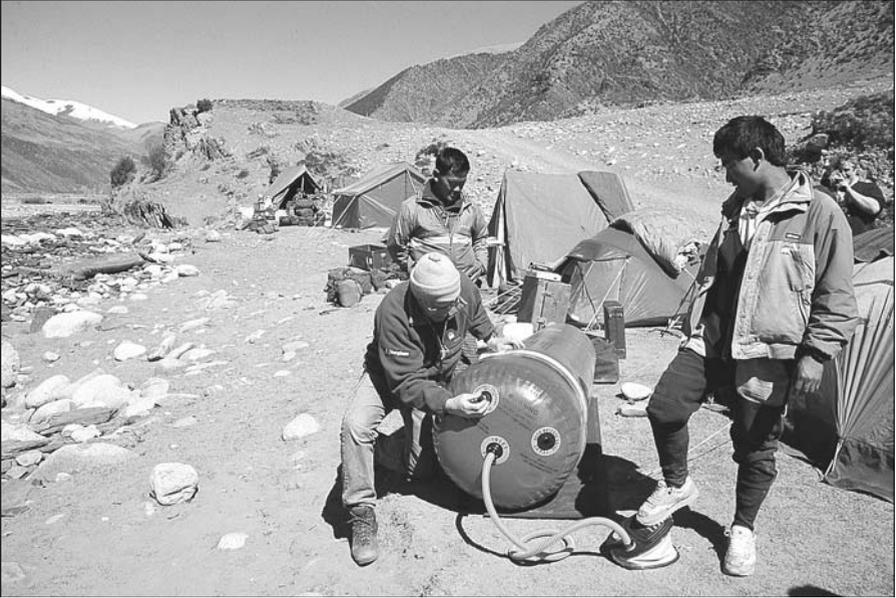
Figure 26.2 *Testing a portable pressure chamber at high altitude – Sepu Kangri Base Camp, 4,700m, eastern Tibet (C. Bonington, Chris Bonington Picture Library)*
