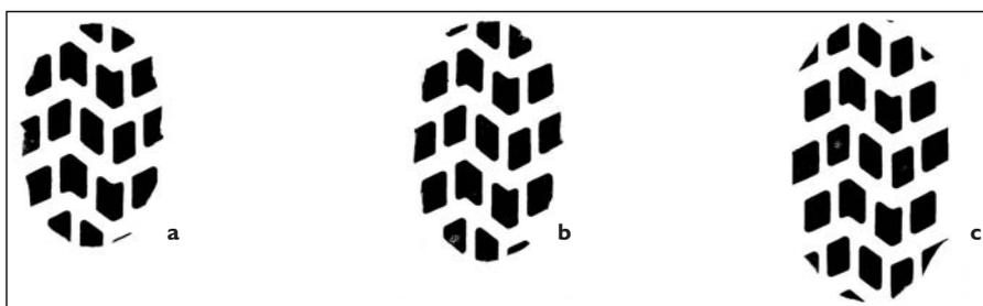
Figure 17.4 Typical tyre footprints at (a) road, (b) track (40 mph maximum) and (c) emergency soft (15 mph maximum) pressures.
