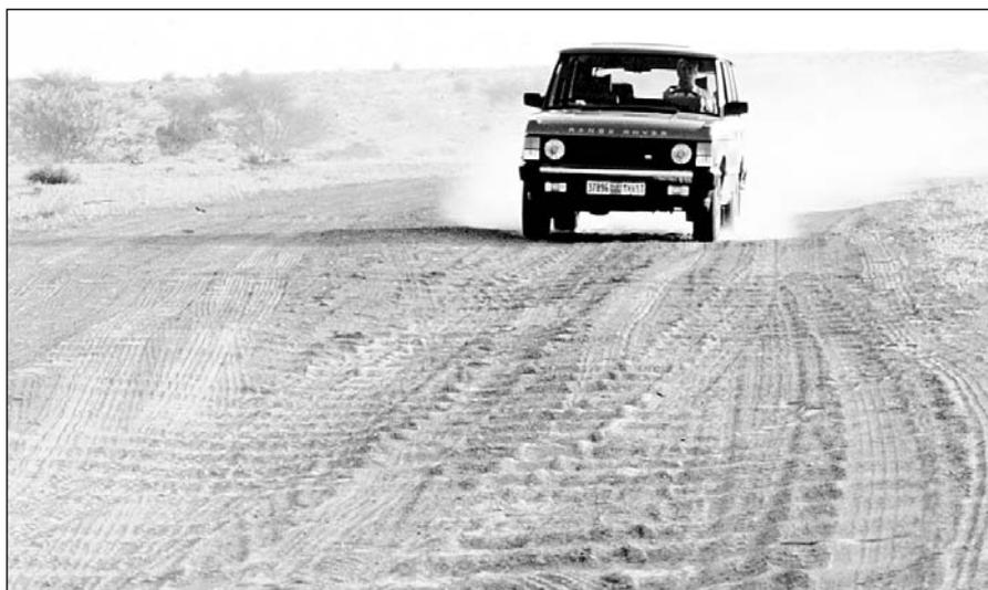
Figure 17.3 *Transverse corrugations are among the most malevolent types of terrain to which it is possible to subject a vehicle. “Track” tyre pressures (see below) are best allied to a “harmonic” speed which transmits less vibration to the vehicle body (© Tom Sheppard)*
