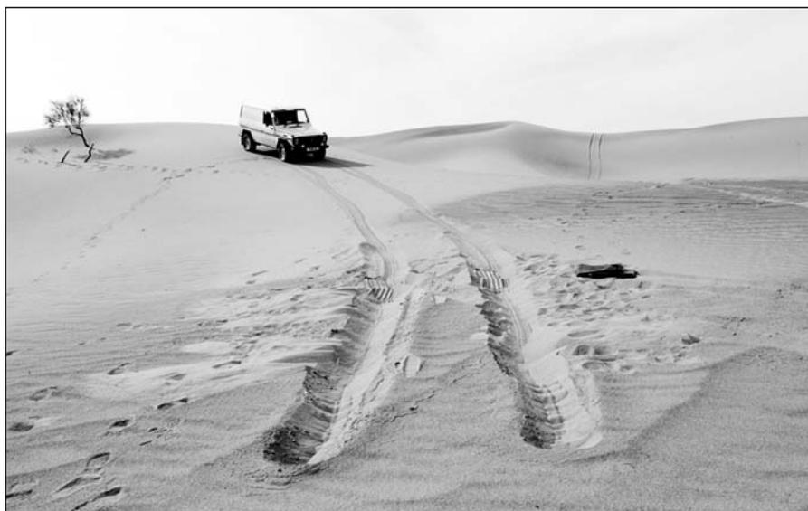
Figure 17.6 *Bogging in soft sand – and de-bogging – soon becomes a standard procedure. Reverse if you can, deflate the tyres to emergency soft, dig sand away from wheels, place sand mats behind rear wheels, reverse back on to firm ground, recce on foot the best way out (© Tom Sheppard)*
