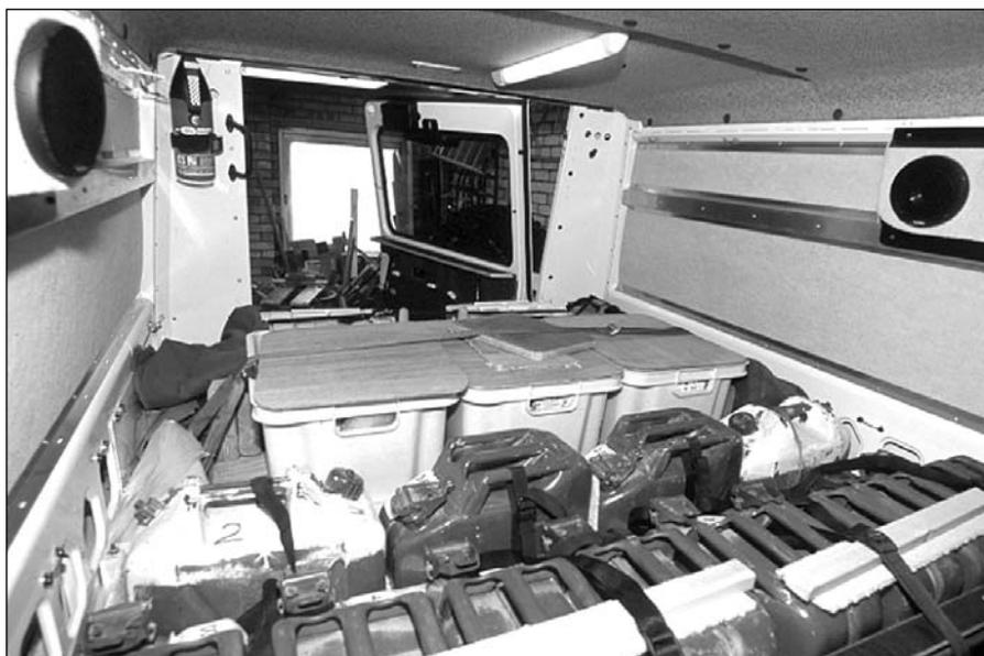
Figure 17.9 *Looking aft from driver's seat, cargo lashed for a desert trip. Fuel and water cans are at the front against the bulkhead; lightweight plastic food storage boxes are lidded and lashed. Note fire extinguisher mounted near back door where cooking takes place (© Tom Sheppard)*
