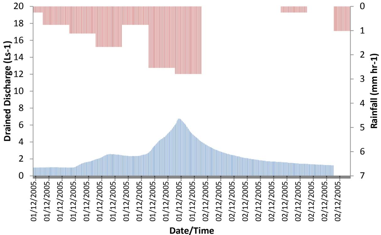
**Figure 3:** River hydrograph plotting discharge through time. Rainfall has been added to allow links to be made between rainfall characteristics and river discharge response.
