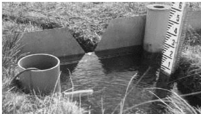
**Figure 1:** V Notch weir used for estimating stage height and discharge (Source: Dr Nick Chappell, University of Lancaster)
