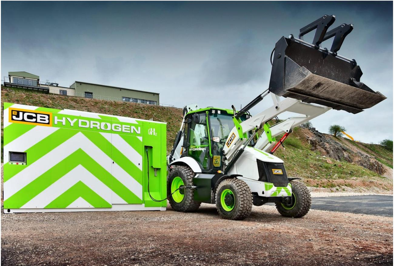
Figure 2 a JCB hydrogen-powered backhoe loader © JCB
