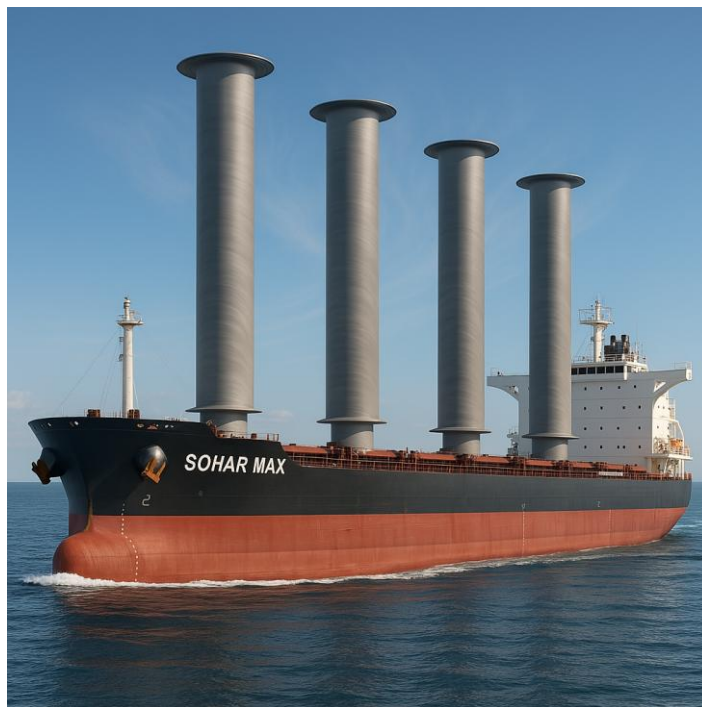
Image: Computer generated image of bulk carrier Sohar Max fitted with rotor sails. Credit: RGS
