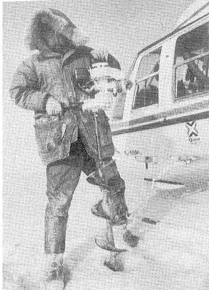
*A powered ice auger is the easiest way to make a hole for ice fishing. Transport by helicopter is an optional extra (courtesy of G. Caron, Fisheries and Oceans Canada, Ottawa).*
